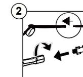
Assemble pressure washer gun to spray wand.
