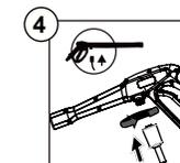
Insert high pressure hose into trigger handle.
